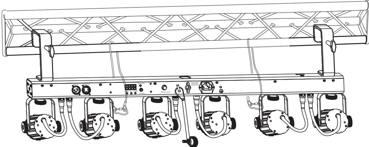
Attach the theatre hooks on the SCY-Bar. Tighten the fixation screws
