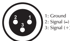
DMX-output XLR mounting-socket:
