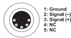
DMX-output XLR mounting-socket:
