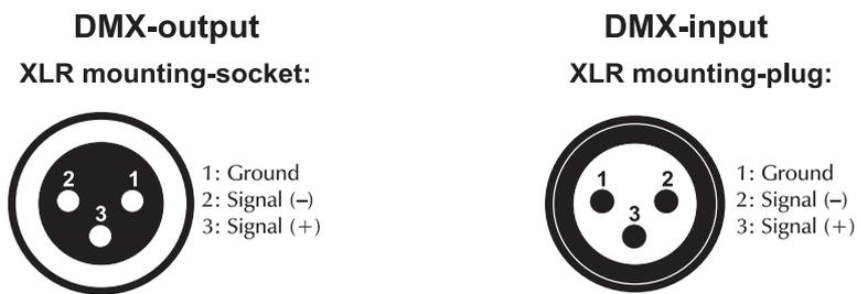
If you are using controllers with this occupation, you can connect the DMX-output of the controller directly with the DMX-input of the first fixture in the DMX-chain. If you wish to connect DMX-controllers with other XLR-outputs, you need to use adapter-cables.
