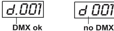
After switching on, the device will automatically detect whether DMX512 data is received or not. If the data is received, the display will show "**d.001**" with the actually set address.
